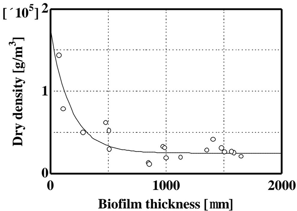
Figure 3.1 Relationship between biofilm thickness and dry density for several biofilm samples (open circles: experimental data; continuous line: smooth curve ( $X = 2.5 \times 10^4 + 1.5 \times 10^5 \cdot \exp(-d/175)$ ))
