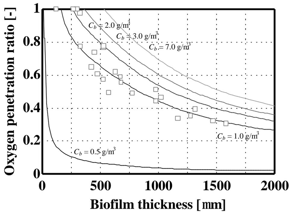
Figure 3.7 Plots of oxygen penetration ratio against biofilm thickness for experimental data obtained at an oxygen concentration of  $1.46 - 2.23 \text{ g/m}^3$  at the biofilm surface. Simulated curves are drawn for oxygen concentrations of  $0.5$  (---),  $1.0$  (- -),  $2.0$  (- · -),  $3.0$  (· · ·) and  $7.0$  (- · ·)  $\text{g/m}^3$  at the biofilm surface
