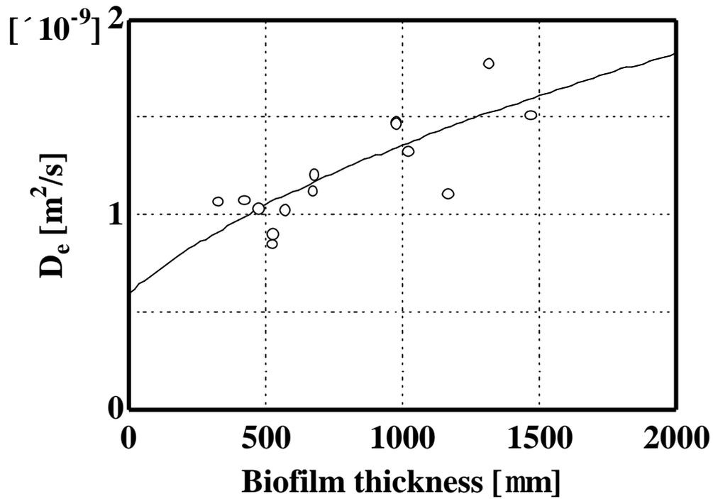
Figure 3.5 Relationship between biofilm thickness and calculated effective diffusion coefficient for several biofilm samples. The empirical equation,  $D_e = (3.5 \cdot 10^{-19} + 1.5 \cdot 10^{-21} \cdot d)^{0.5}$ , is shown as a continuous line
